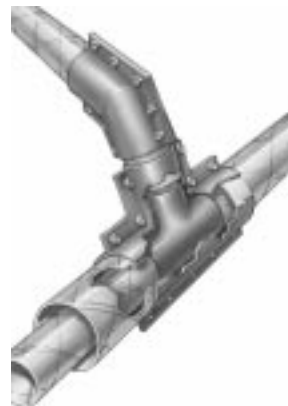
Figure 4 - Example of FRP Double-Walled Piping
